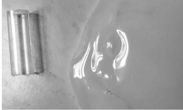
Figure 12.6 Same material, two different cooling rates (left: fast cooling rate; right: slow cooling rate)
