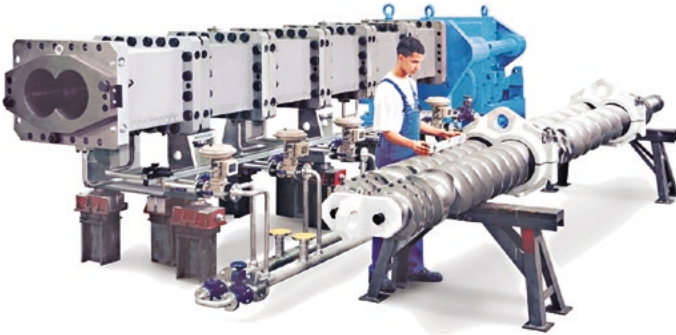
Figure 1.11 Barrel and screw configuration sequence for homopolymer powder to pellet conversion (courtesy of Coperion Corporation)
