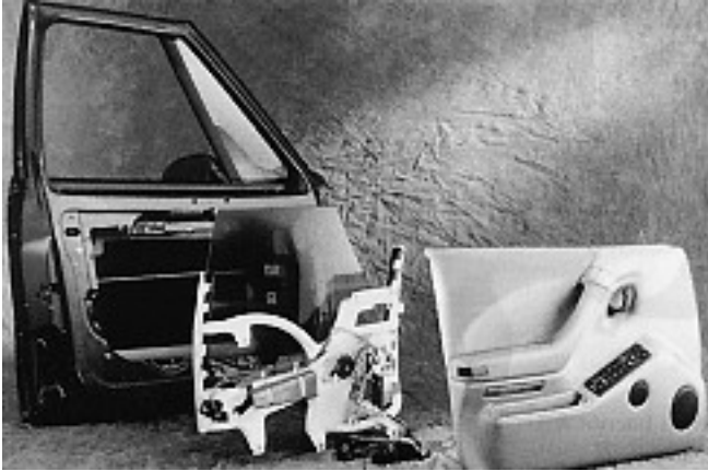
Figure 1.21 Delphi Interior & Lighting Systems door module in place [From Injection Molding Alternatives , Avery, J. (1998)]
