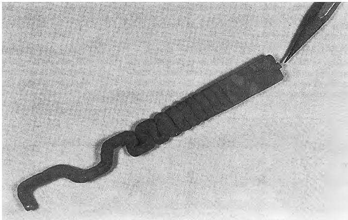
Figure 2.35 When jetting does occur, the parts have poor surface appearance due to improper welding of the jetting melt as the cavity fills. Jetting can also result in a reduction in mechanical performance
