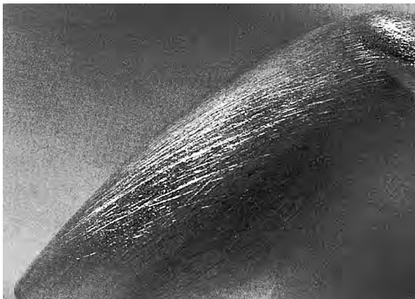
Figure 3.28 Photo showing craze formation on an acrylic part
