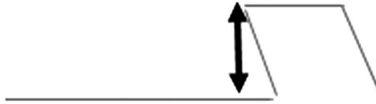
Figure 1.7 Measuring flight depth in metering section
