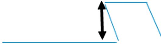
Figure 1.7 Measuring flight depth in metering section
