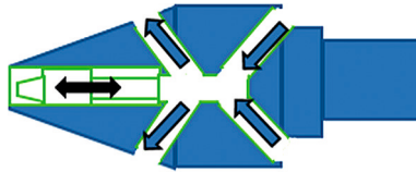
Figure 1.13 Flow through a poppet tip (cut away)
