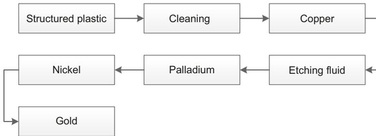
**FIGURE 3.28** Flowchart for beaker metallization
