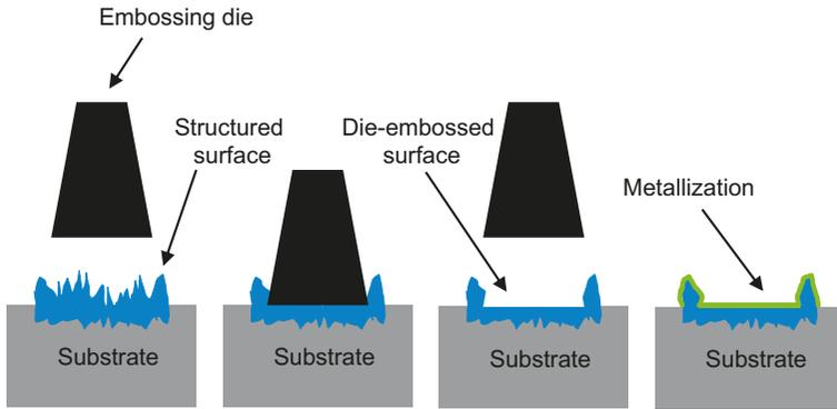
**FIGURE 3.29** Diagrammatic illustration of smoothing by die embossing as in [185]
