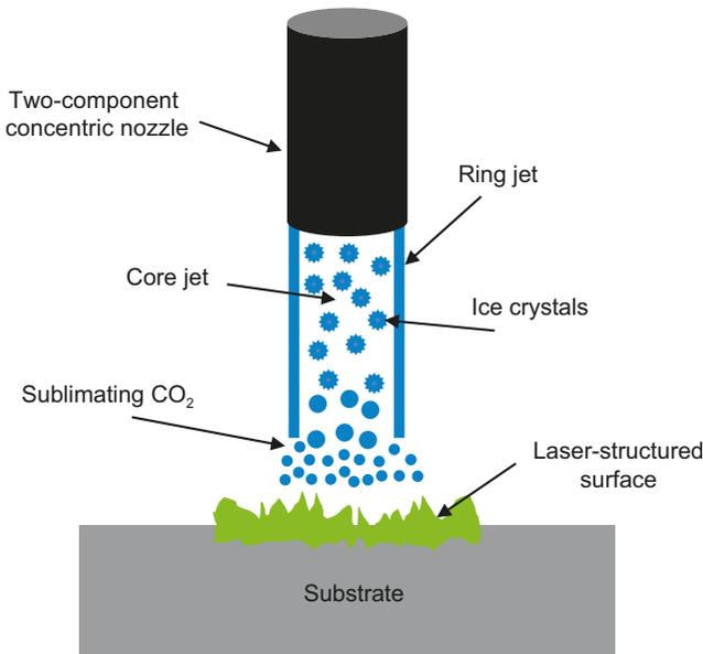
**FIGURE 3.31** Diagrammatic view of CO<sub>2</sub> snow-jet smoothing as in [1]
