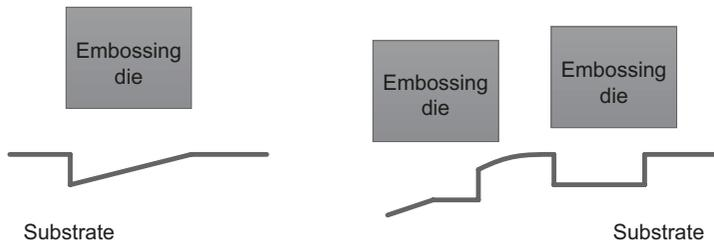
**FIGURE 3.30** Possible faults due to lack of parallelism as in [185]
