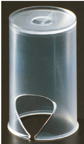
Figure 6.30 Center-gated canister molded in a 16-cavity hot runner. Asymmetric melt conditions resulted in the intra-cavity filling imbalance shown
