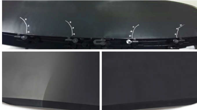
Figure 11.25 Automotive part where the left side was molded with a traditional fast-opening valve gate versus the right side that was molded using a profiled servo driven valve gate (Courtesy: HRSflow)
