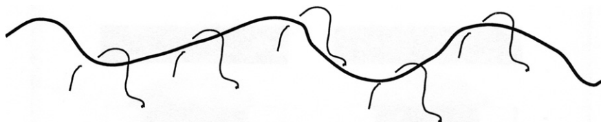
Figure 7.1 Illustration of a long polymer (artificially straightened for illustrative purposes) entangled with much shorter chains, where the long-chain concentration is too low to permit entanglements between long chains
