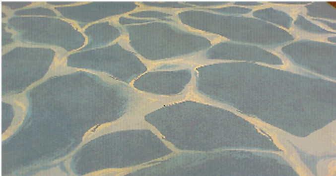
Figure 1.11 Sketch of the Cross-Dual-Phase entanglement network model. The boundaries of the “white phase” are not static but fluctuating around with frequency \omega'_0 under no stress conditions. Stress increases the frequency of reorganization and, in the rubbery plateau region, preferentially orients the boundaries in the flow direction. This can be modeled by an activated process
