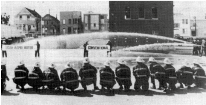
Figure 1.11 Effect of drag reduction on fire hose range (Taken from Schowalter, 1978, with permission)
