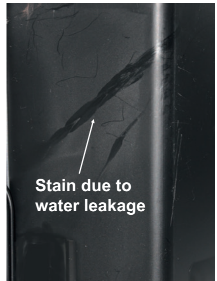
Figure 29.24 Here there is a diagonal mark on the surface that was formed when plastic melt came in contact with water in the cavity.
