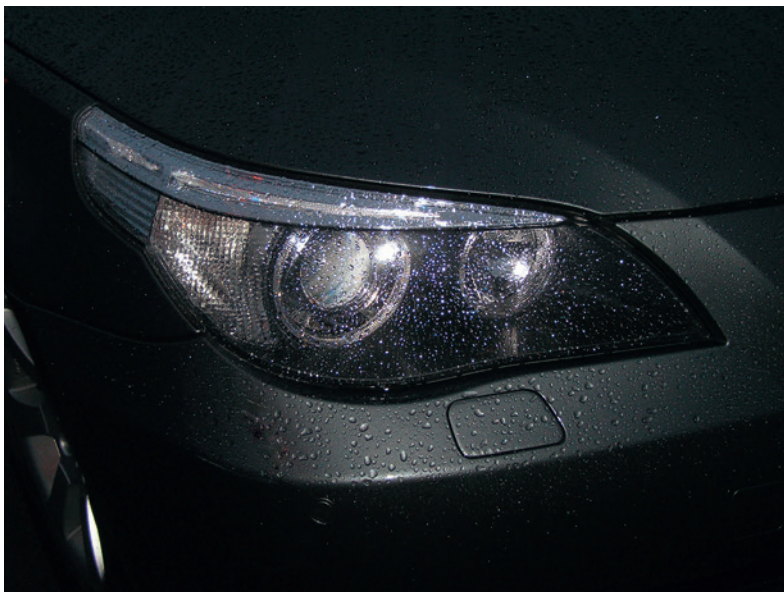
Figure 3.28 The glass for car headlamps is made of polycarbonate and coated with a thin layer of siloxane to improve scratch resistance, UV protection, and protection against solvents.
