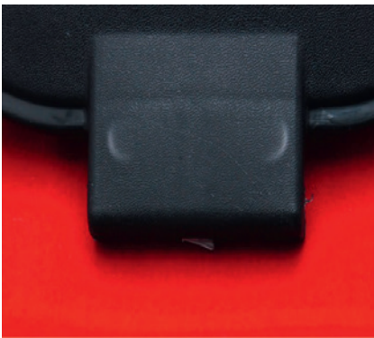
Figure 29.22 Here there are visible ejector pin marks looking like white crescent moons. You can also see a clear sink mark.
