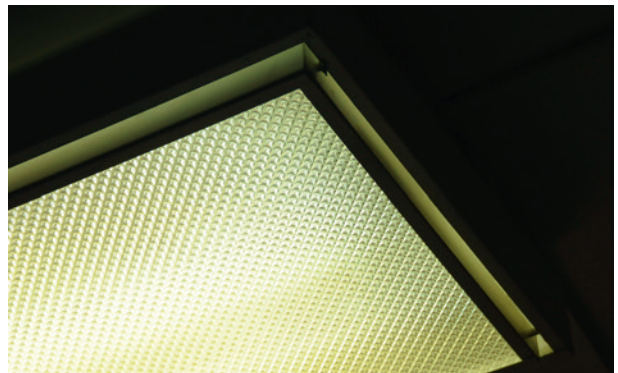
Figure 2.28 PMMA is much used by the lighting industry, e.g. as a screen for fluorescent tubes.
