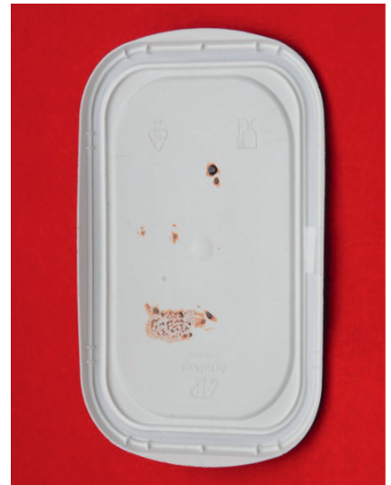
Figure 29.23 Here there are brown greasy oil stains on a white plastic cap.
