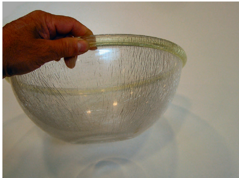
Figure 3.26 Polycarbonate has a poor chemical resistance, as can be seen from the cracks caused by vinegar in the salad bowl here.
