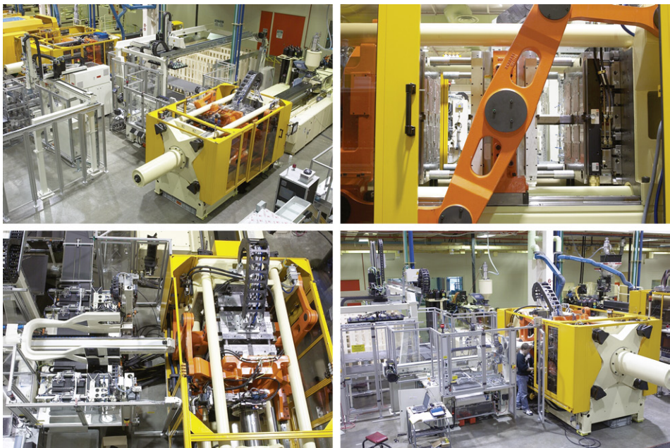
Figure 1.3 Fully automated injection molding work cell for DVD cases, containing 16 components in the work cell (Courtesy of Husky Injection Molding Systems Ltd.)
