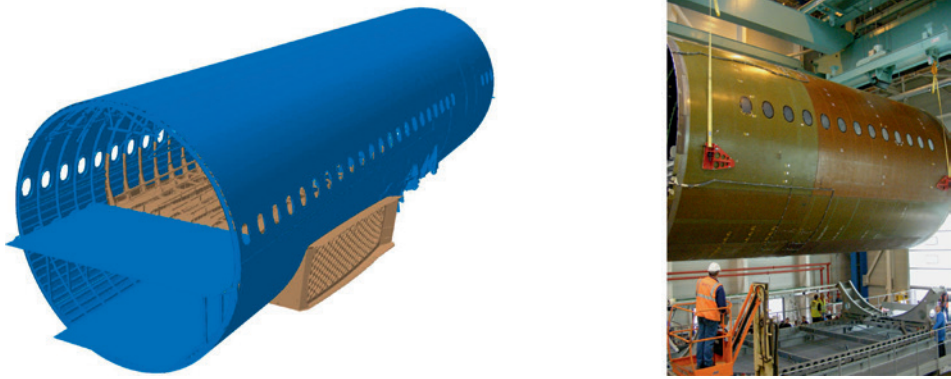
Figure 4.16 Carbon fiber reinforced composite fuselage structures [Courtesy: Airbus Operations GmbH]
