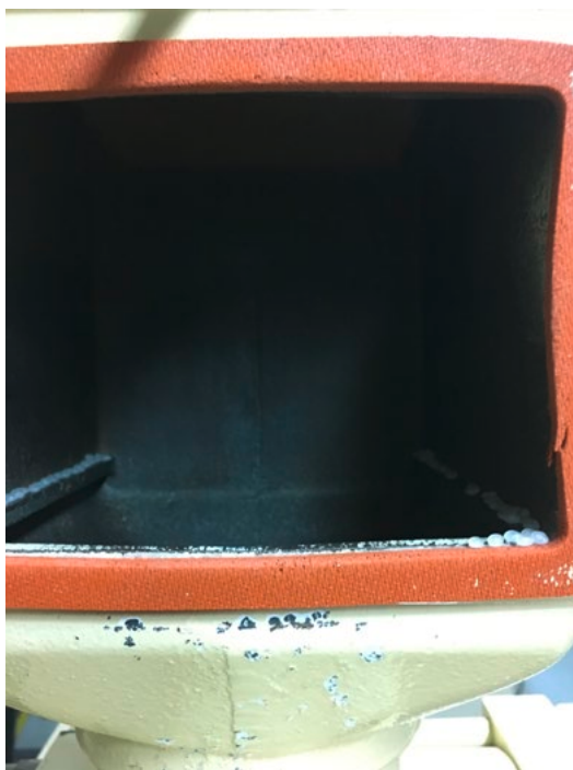
Figure 23.2 Pellets stuck in magnet drawer
