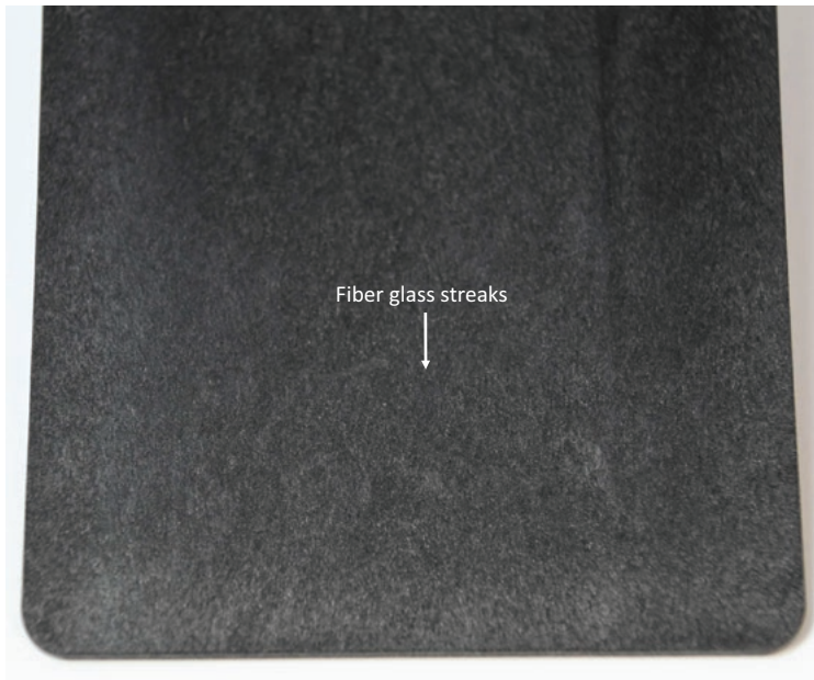
Figure 1.21 Glass fiber streaks
