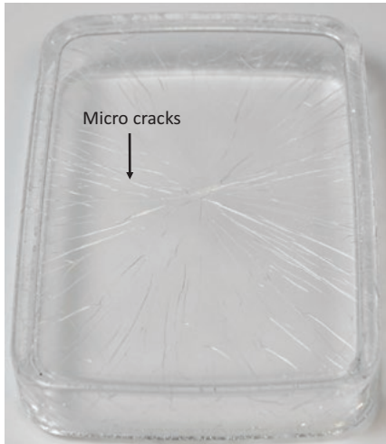
Figure 1.25 Formation of stress cracks, micro cracks
