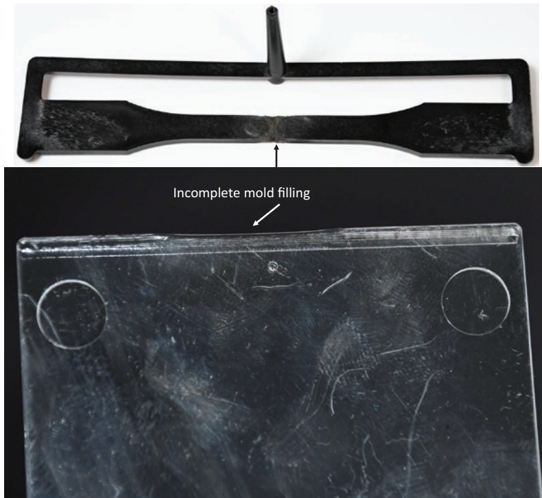
Figure 1.19 Incomplete filling of the tool
