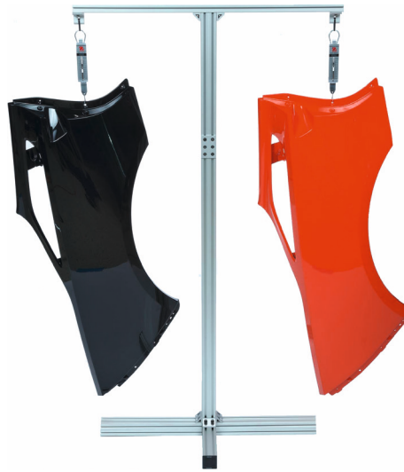
Figure 1.15 Passenger side rear quarter panel for Chevrolet Corvette C7, fabricated by Continental Structural Plastics, a Teijin Holdings USA company, using Class A compatible TCA (Tough Class A) ultra lite sheet molding compound reinforced with 3M iM16K glass bubbles (Courtesy of 3M Company)
