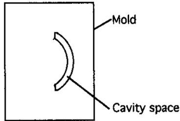
Figure 4.1 Illustration of basic mold, with one cavity space.
