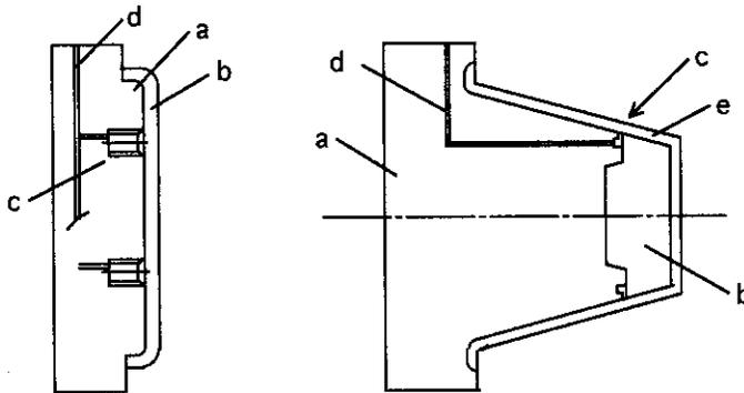
Figure 4.10 Air ejection alone. (Left) (a) core and mounting plate, (b) molded product, (c) air valves, (d) pressure air supply. (Right) (a) core and mounting plate, (b) core tip, (c) circular air gap, (d) pressure air supply, (e) molded product.
