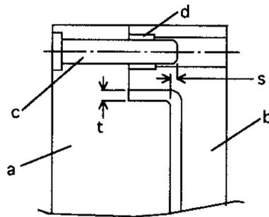
Figure 4.11 Typical mold with leader pin and bushing alignment: (a) core plate, (b) cavity plate, (c) leader pin, (d) leader pin bushing, (s) safety distance of pin above core, (t) wall thickness of plastic product at parting line.
