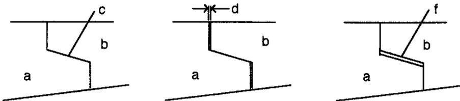
Figure 4.12 Taper (or wedge) lock: (a) male member, (b) female member, (c) taper. (Left) Ideal condition. (Center) Correct application.  $d$  is called preload. (Right) Useless taper.
