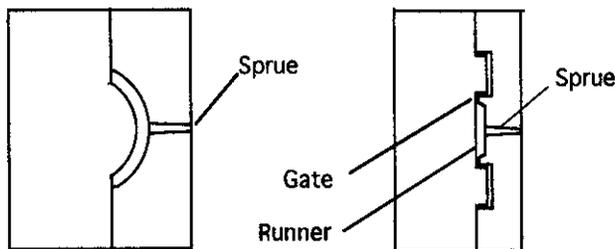
Figure 4.5 Illustration of schematic mold, showing cold sprue (left) and cold runner (right).
