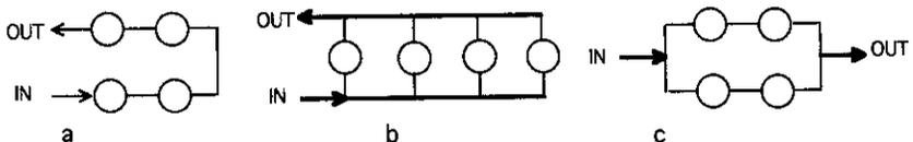
Figure 4.7 Schematic layout of (a) series cooling, (b) parallel cooling, and (c) series-parallel cooling.
