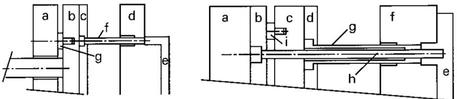
Figure 4.8 (Left) Section through ejector pin mold: (a) backing plate, (b) ejector plate, (c) ejector retainer plate, (d) core plate, (e) molded product, (f) ejector pin, (g) stop pin. (Right) Section through sleeve ejector mold: (a) backing plate, (b) core pin retainer plate, (c) ejector plate, (d) sleeve retainer plate, (e) molded product, (f) core plate, (g) sleeve ejector, (h) core pin, (i) stop pin.
