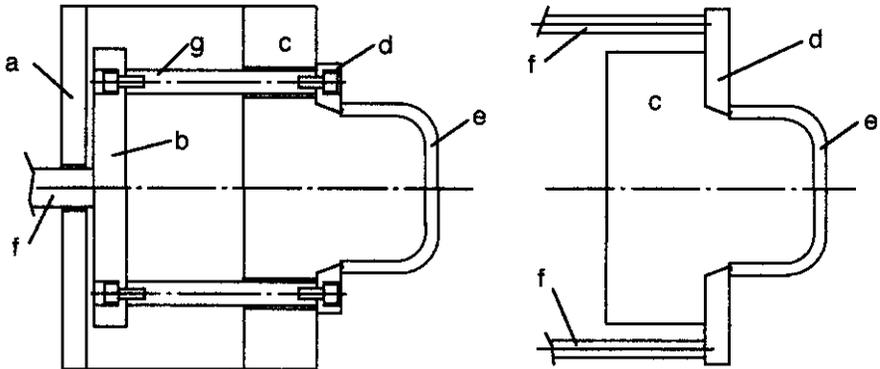
Figure 4.9 (Left) Section through stripper ring mold: (a) mounting plate, (b) ejector plate, (c) core plate, (d) stripper ring, (e) molded product, (f) machine ejector, (g) connecting sleeve. (Right) Section through stripper plate mold: (c) core and mounting plate, (d) stripper plate, (e) molded product, (f) machine ejectors.
