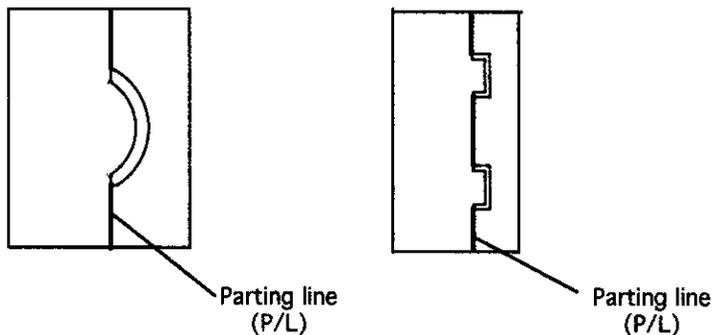
Figure 4.3 Illustration of schematic mold, showing the parting line.
