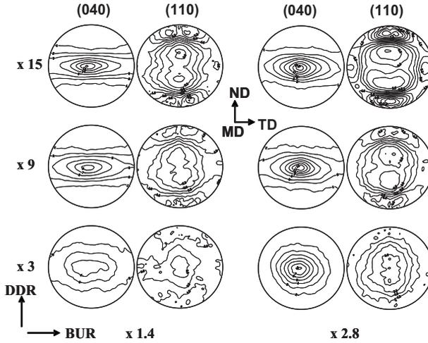
Figure 9.16 Typical pole figure patterns for isotactic polypropylene tubular blown films (D. Choi and White [72])
