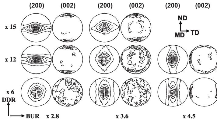
**Figure 9.18** Typical pole figure patterns for syndiotactic polypropylene tubular blown films (D. Choi and White [72])
