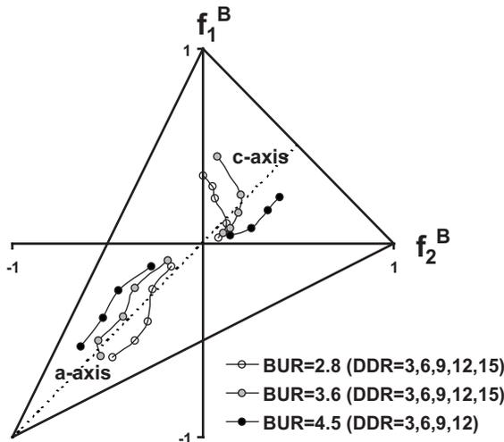
**Figure 9.19** Biaxial orientation factors of syndiotactic polypropylene tubular blown films (D. Choi and White [72])
