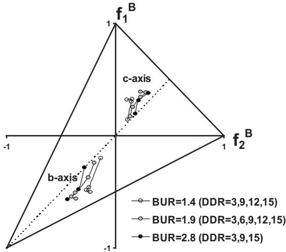
Figure 9.17 Biaxial orientation factors of isotactic polypropylene tubular blown films (D. Choi and White [72])
